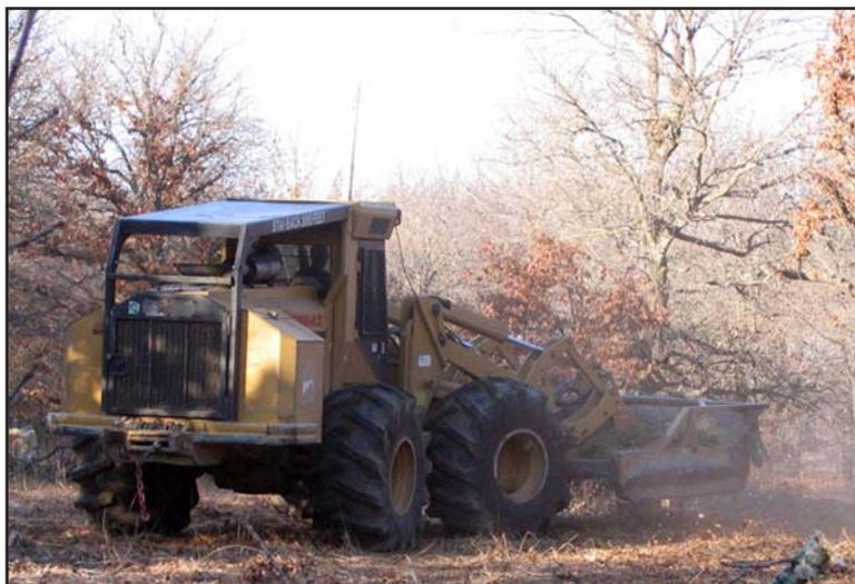
"The Hydro Ax machine can clear eight feet in a single pass, cutting brush and trees up to 10-inches in diameter," says Roger McAllister, IEC's right-of-way supervisor.
